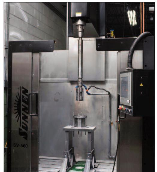
The SV-560's powerful 60-inch (1524 mm) stroke finishes holes up to 9-inch (228.6 mm) diameter.
