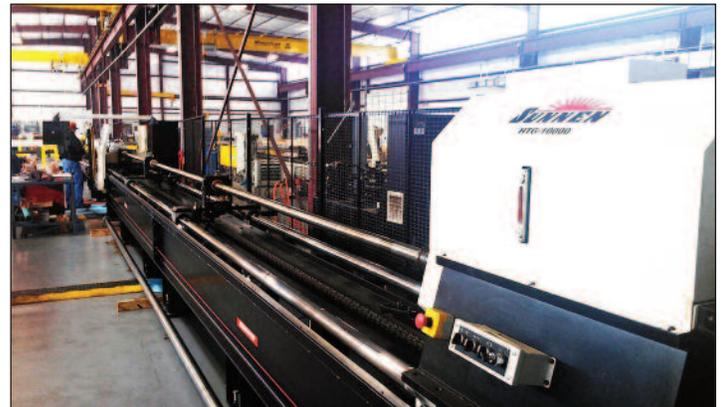
Hole Specialists' new HTG-10000 tube hone with a 32-foot (10 m) stroke and I.D. capacity of 24 inches (610 mm), is "big" even by Texas standards.
