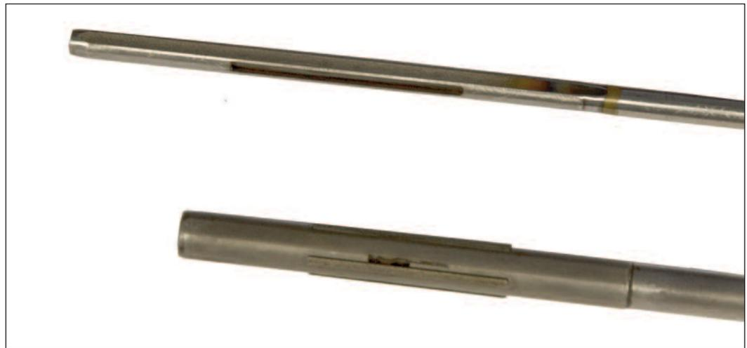
Sunnen LBT tools for gun barrels are available in diameters from 0.168" to 0.500" (4.27 - 12.7 mm). They carry 2, 3 or 4 superabrasive stones (CBN or diamond) of varying length and width, depending on the tool's diameter. The tool is made of thru-hardened tool steel, and the stones are field-reloadable. Larger diameter tools can be custom-ordered
