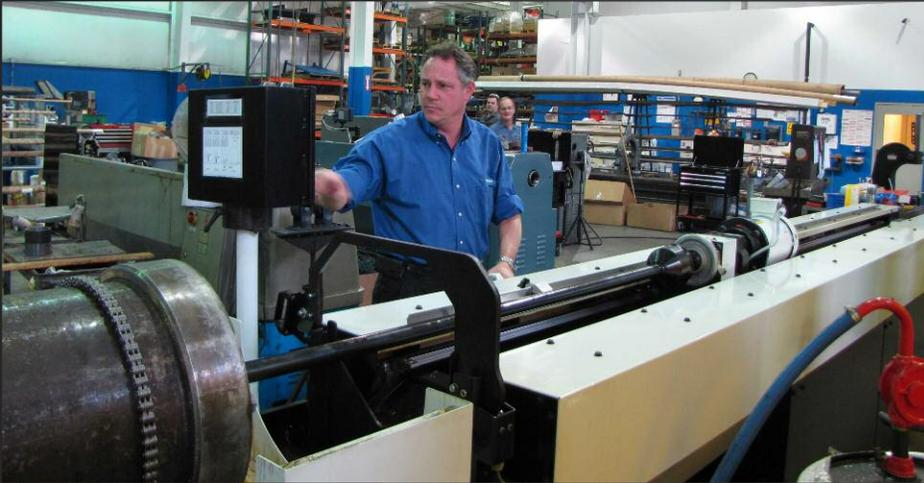
Air Hydro's Perry Goldstein sets up a Sunnen HTA tube hone to recondition a hydraulic cylinder. The HTA includes a Siemens drive and PLC control with touch-screen HMI for setting machine parameters such as stroke reversal point, spindle/stroking speed and crosshatch angle calculation.
