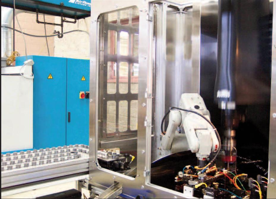
A two-position rotary table with automated part loading by servo robot allows high-volume processing in unattended mode, while holding tolerances as tight as 0.000050 (1.25 μm). Protective doors removed from front of machine for photos.
