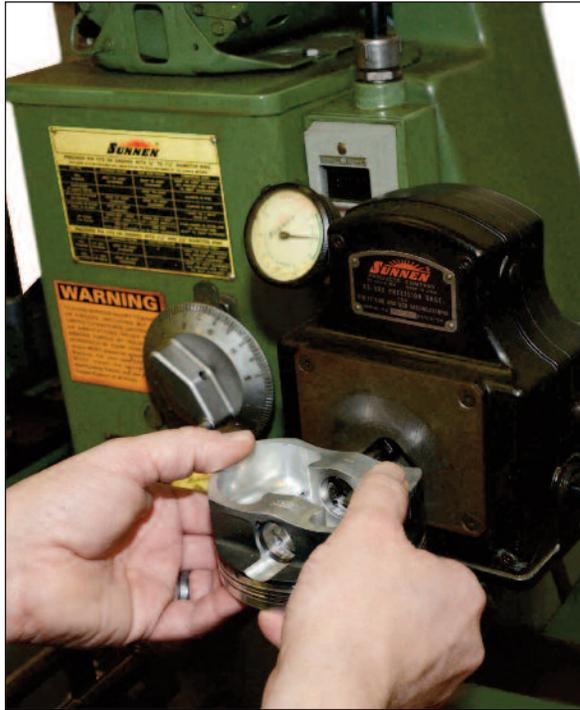
Piston pin bore is measured on a Sunnen AG-300 gage after honing on an older LBB model machine.
