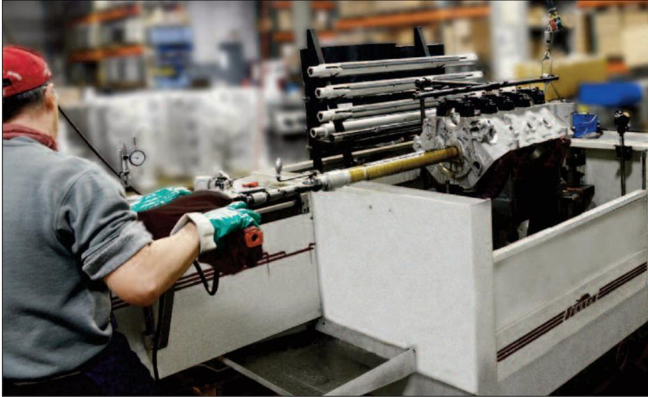
A Sunnen CH-100 fixtures a block for manual honing of the cam tunnel.
