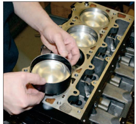
A ring compressor eliminates pre-compression of the rings and insures square installation in the bore.
