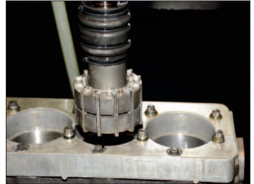
Sunnen's two-stage diamond abrasive honing tool does roughing and finishing with 220- and 500-grit abrasive without pause for stone change. The advanced control system on the SV-20 allows Dart to achieve a wide range of finishes with these two abrasives.
