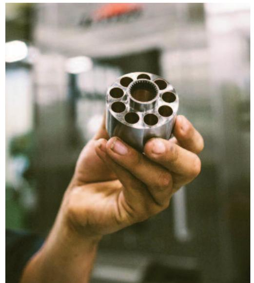
The heart of a hydraulic piston pump, called a cylinder block or rotor, starts as a turned blank up to eight inches diameter. Then, nine circumferential piston bores from 0.1875" to 1.5" (4.8 - 38.1 mm) diameter are roughed in on a machining center, and the part may be heat treated.
