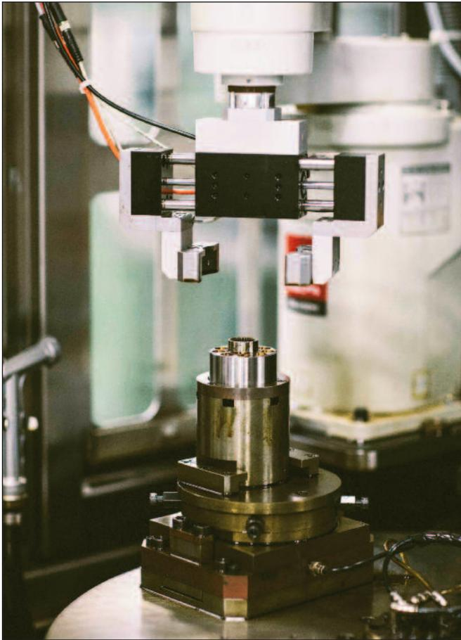
After each bore is honed and air-gaged as acceptable, a robot inside the honing machine's work envelope rotates the workpiece to align the next bore for the honing tool
