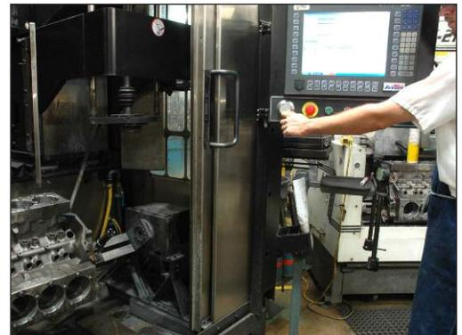
Setup is simplified with a multi-axis hand wheel for fine-tuning vertical stroke, tool feed, column position and optional cradle position. The fully automated system indexes the tool from bore to bore and (for V-blocks) the servo fixture rolls the block for access to all cylinders, ending with a rollover of the block to dump oil/coolant.
