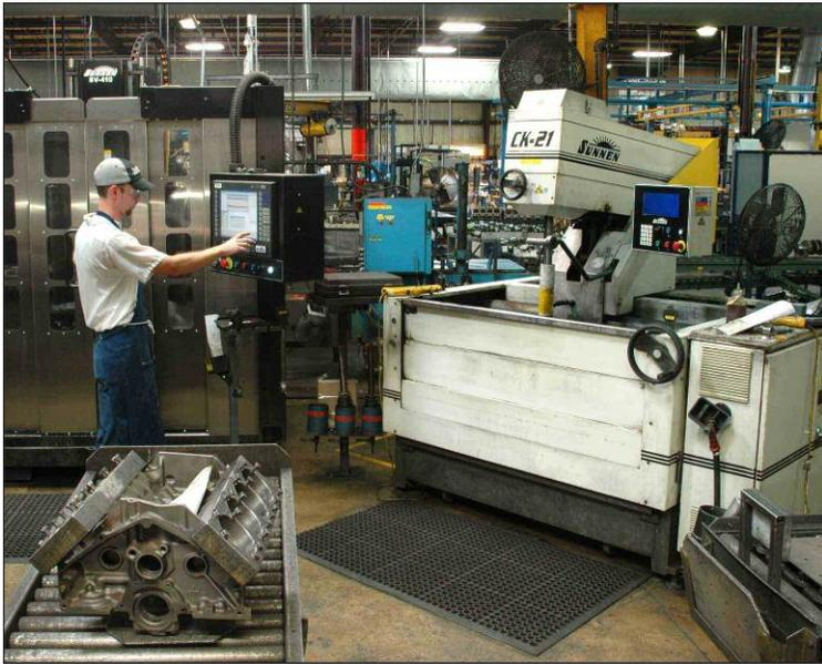
The honing operator simply tells the control what block is in the fixture and what the oversize should be, then hits cycle start. The honing machine senses the size and knows what to do to produce the finished bore while the operator tends the CK-21 machine
