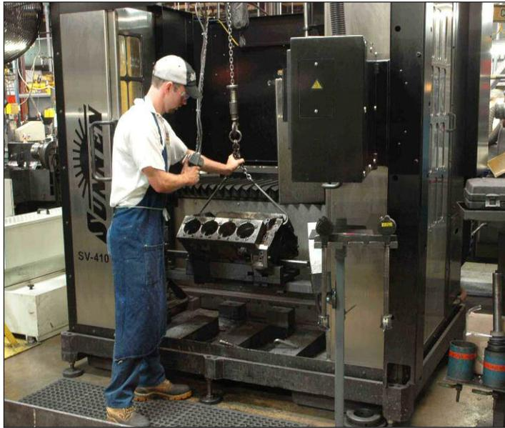
The SV-410 features full-height/walk-in access doors and stainless steel enclosure to ease part load/unload and improve maintenance.
