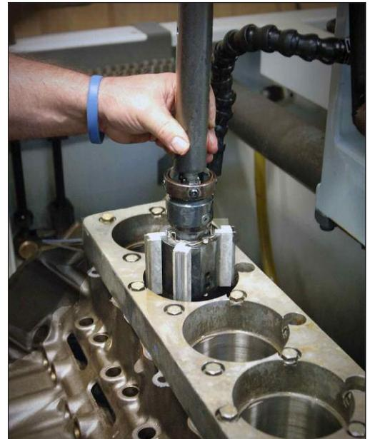
Sunnen DH diamond hone head provides multipoint abrasive contact on the bore and a cone-style feed system produces uniform feed pressure on the circumference of the tool for exceptional roundness. White's original set of abrasives lasted 18 months.
