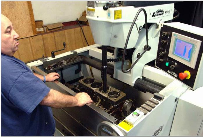
A patented full-bore profile display on the SV-10's control shows a real-time cross section of the bore, which takes the guesswork out of removing taper.
