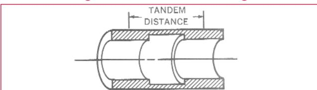
Tandem distance is the center to center length of two bores, as shown.
