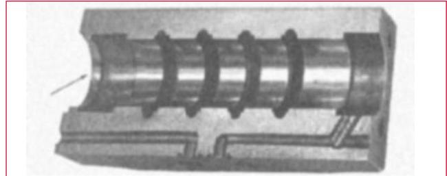
The narrow land indicated by the arrow (left) would have a tendency to go a few tenths oversize if it were stroked and reversed the same as the other lands in this valve body. Its smaller surface area is honed faster than the wide lands. As final size is reached, the part should be honed from the right end, with the narrow land only occasionally overstroked as needed to bring it to size and alignment.
