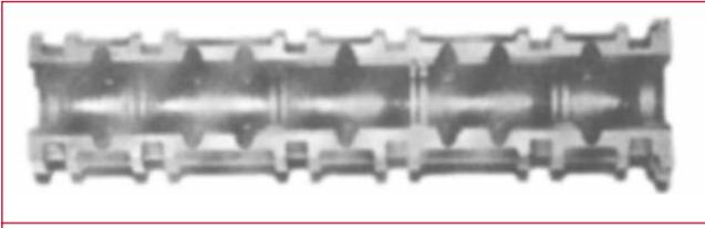
Note the six narrow lands widely spaced. Not only must the multiple bores be of exact diameter, but they must also be exactly in line.
