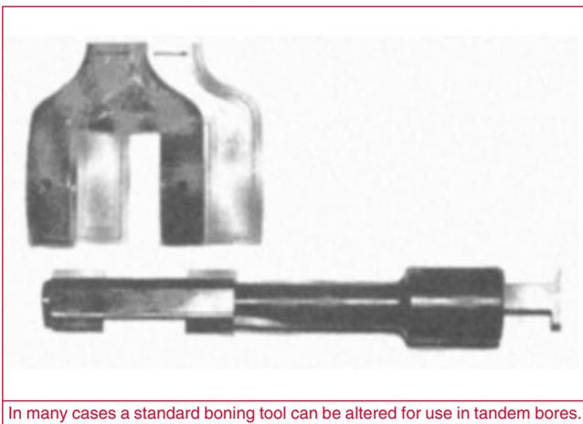
In many cases a standard honing tool can be altered for use in tandem bores.
