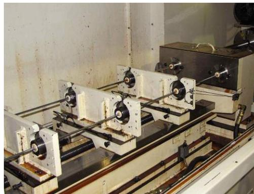
Feddersen's patented whip guide stabilizers used on DeHoff gun drill.
