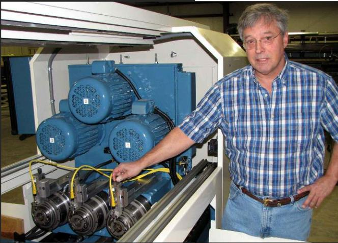
Fred Feddersen shows off a part presence sensing system he devised for his new gun drilling system.
