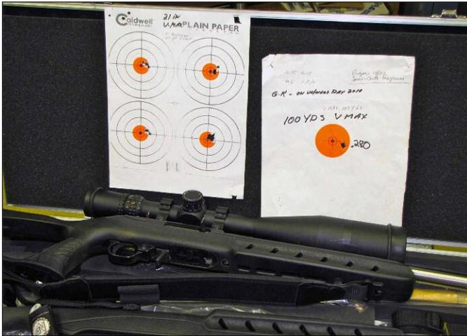
A series of targets with a pair of Ruger .22 magnum semiautomatic rifles equipped with Feddersen barrels. Targets on left are five shots each at 50 yards. Target on right is five shots, 100 yards.
