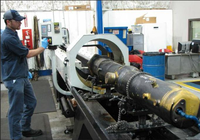
Caterpillar dealer Wayne Supply has honed hydraulic cylinders up to 21 feet long, saving customers 80 percent over the cost of a new barrel.
