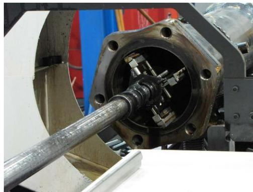
The HTA hone is designed for optimum performance with Sunnen ANR275 tooling and abrasives, sold with matching coolants and gauging as part of the machine package.
