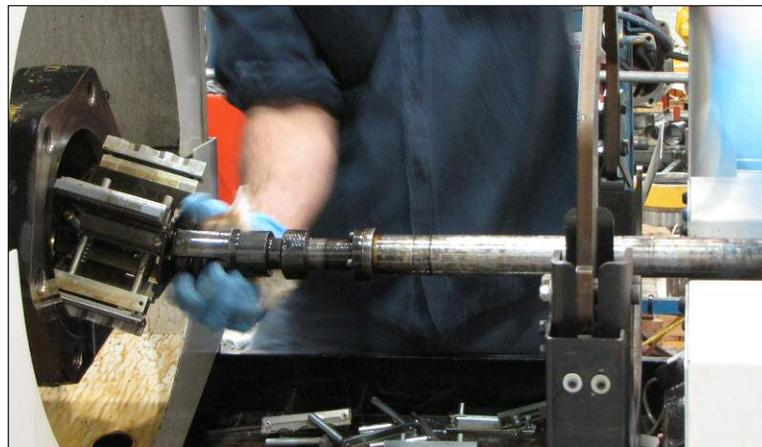
Whayne honing operator changes abrasives to perform both roughing and finishing of the bore.
