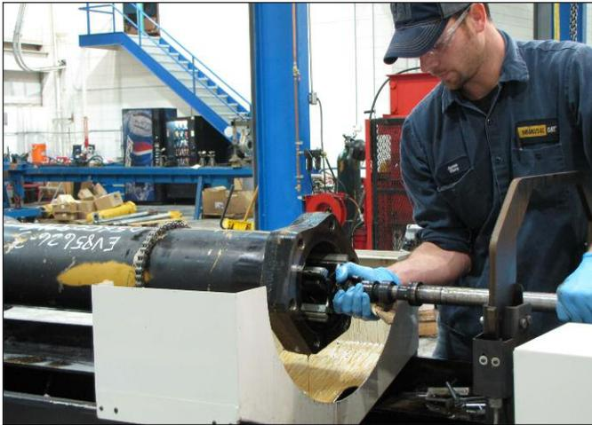
Whayne honing operator inserts the tool at start of a cycle. Whayne has honed cylinders with bore ID up to 17 inches. The HTA tube honing system handles parts weighing up to 8,000 lbs. (3629 kg) with ID ranges from 2.5 inches to 21 inches (63.5 to 533 mm).
