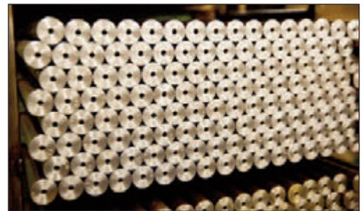
**Pac-Nor cuts and faces premium bar stock, then gun drills on one of five twin-spindle machines, followed by reaming of the blanks. This rack of barrel blanks awaits completion.**
