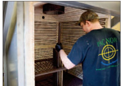
At Pac-Nor, barrel blanks are stress relieved in a tempering furnace after honing and rifling. The parts are inspected and gaged at various stages during manufacture.
