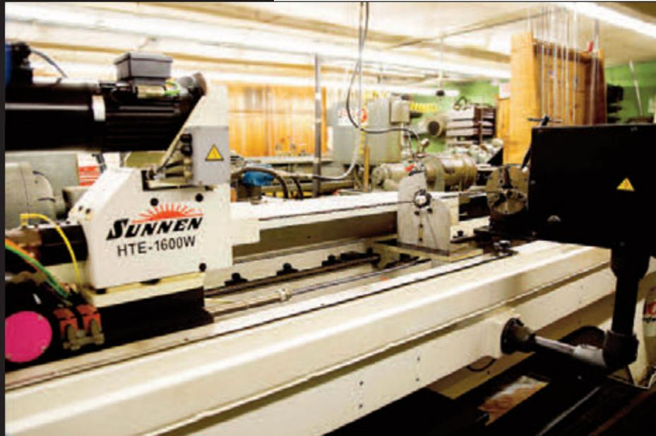
Pac-Nor Production Manager Casey Dichter says the Sunnen hone produces a consistency in bore diameter that is head and shoulders above lapping. The machine has all but eliminated the standard pre-rifling lap.
