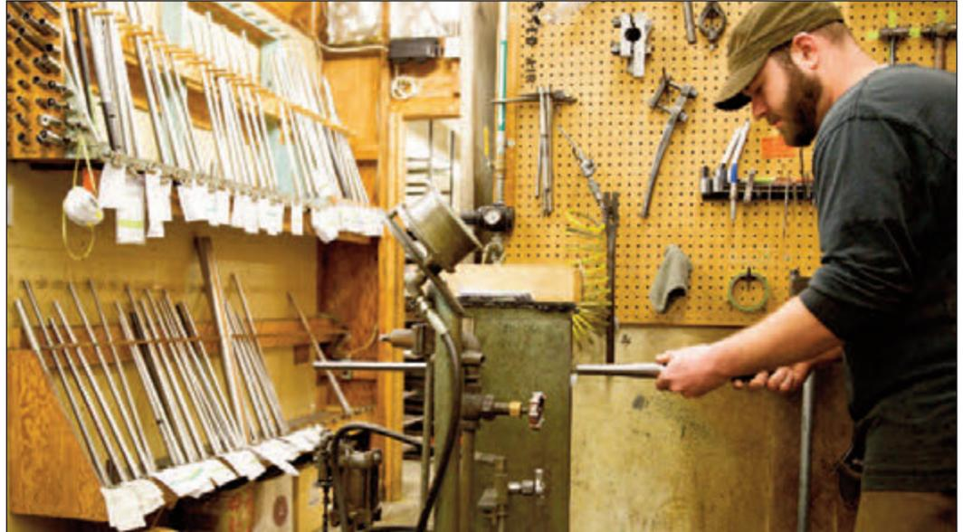
**Maverick McCourt prepares to install a rifle barrel on a receiver using Pac-Nor's barrel press.**
