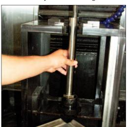
Sonic's fuse pins have various diameters and lengths up to 23 inches. The Sunnen SV-1000 handles diameters up to 3 inches and stroke lengths to 31 inches.
