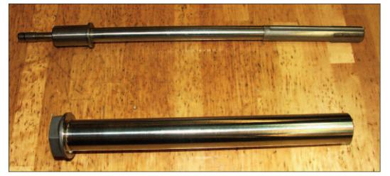
Sonic Industries must meet ID tolerances of 5 to 7 microns, with a surface finish in the range of 8-16 RMS, for its fuse pins. The pins attach jet engines onto the wing and break away in emergency situations to prevent catastrophic structural damage and/or fires.
