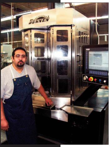
Sonic used to hone fuse pins manually; the CNC-controlled SV-1000 helped reduce cycle times by 75 percent, and increased productivity from nine to 40 parts per day
