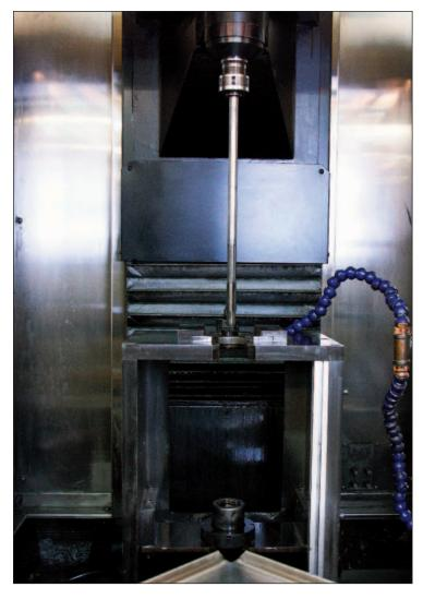
Sonic uses Sunnen MMT superabrasive tools, which last five times longer than conventional designs and can reduce per-part cost by 30 percent.
