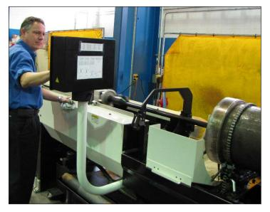
A touch-screen controlled hone provides a safer working environment and reduces operator fatigue, as well as providing better quality parts by producing a controlled crosshatch pattern, which allows the honed surface to retain oil or grease and ensure proper lubrication.
