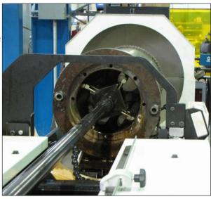
Adding the HTA to its repair shop machine tool lineup allowed Air Hydro to bring previously farmed honing work back in-house, helping it regain control of job turnaround times and save money on outsourcing.
