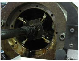
The Sunnen HTA tube honing system handles parts weighing up to 8000 lbs (3629 kg) with ID ranges from 2.5 inches to 21 inches (63.5 to 533 mm), and is available for 6-foot (2m) and 12-foot (4m) part lengths.
