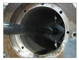
Transition to the HTA was easy for Air Hydro Power: the machine uses the same Sunnen ANR tooling the shop was using to hand hone.
