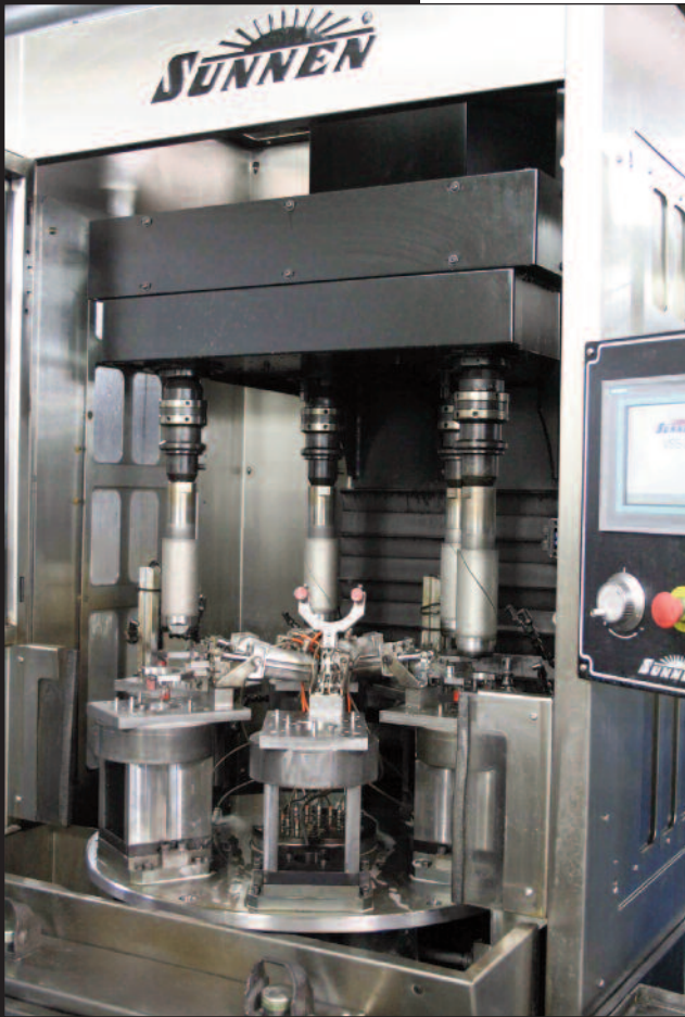
4-spindle VSS-2 honing system used by Cloyes Gear to hone the bores of VVT stators. The segmented bore of the powder metal parts is finished to a roundness of 50 microns and total tolerance of 80 microns.
