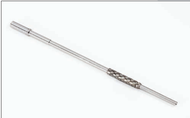
Custom designed lapping arbor and sleeve (left). Closeup of SVL-2115 fixture with lapping tool.
