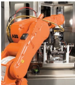
A TWO-AXIS OR MULTI-AXIS SERVO ROBOT CAN BE INTEGRATED INTO A SUNNEN MODULAR SYSTEM.
