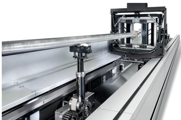
The **optional workpiece supports** retract automatically, designed to support small diameter parts. Up to 3 supports are possible.
