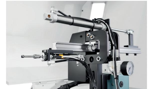
The **in-process plug gauge** is reliable and independent of stone wear in holding tightest tolerances. The long-life carbide probe controls on reverse stroke with an accuracy of up to 0.002 mm.
