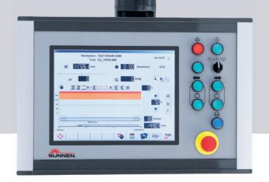
**Intuitive touch control** with clear, self-explanatory screen. It is the ideal system for optimized process control and fits in all production industries. No programming skills required. A new set-up can be made within 2 minutes, step-by-step. The system recommends the required tool, sets the spindle speed and all necessary cycle parameters. All parameters can be stored.
