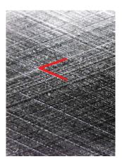
The new Sunnen2 controls on the SV-35 allow for a consistent crosshatch surface finish from the top to the bottom of the bore.
