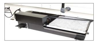
Standard dual filtration 55-gallon capacity manual paperbed filter which is easily accessable from the front of the machine.
