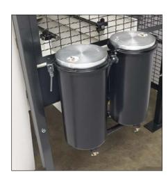
The additional standard dual cartridge filter ensures clean honing fluid for demanding processes.
