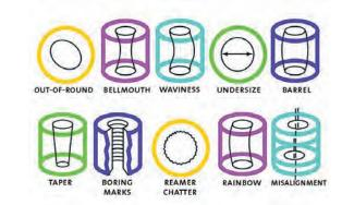
There are ten common bore errors that are caused by machining, heat treat or chucking. All of them can be corrected quickly and easily on the Sunnen MBB-1660.
